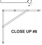
On the other side attach both ends of the Special **Bottom Support Channel** to the Support channels. Drill hole through both Support Channels and attach with nut and bolt.
